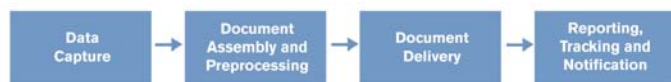
Figure 3: RightFax incorporates a four-phase process that captures any form of information, renders it into an electronic image, distributes the information via fax, email or over the Internet and creates customized reporting, including host notifications.
